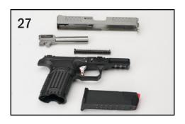
13. Your AXE pistol is now disassembled (field stripped) and ready to be cleaned.
