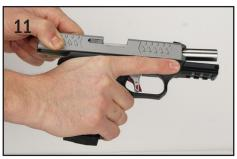
3.Lock the slide in the rearward position by pushing up on the slide stop lever (27) and slowly release the slide from the fully rearward position until it locks in the open position.
