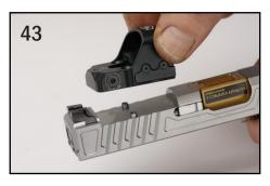
3.Using the appropriate screws that were provided with your optic sight, tighten the side down onto the slide. (picture 44-45)
