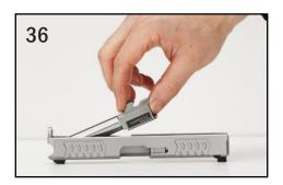
2.Insert the recoil spring assembly (3) into the slide by placing the small end of the recoil spring assembly in the indentation in the front of the slide and pressing the other end of the recoil spring assembly towards the front of the slide to compress the spring and pushing down until the large end of the recoil spring assembly rests in the second (semi-circular) notch on the barrel locking cams (Pictures 37-39).
