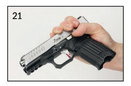
8.Using your fingers, retract the slide (1) about 1/8 in. / 3mm and hold it in this position (Picture 22). (Note: If you pull the slide too far to the rear, it will reset the pistol's trigger to the forward position. If this happens, pull the trigger again while keeping the muzzle of your firearm pointed in a safe direction.
